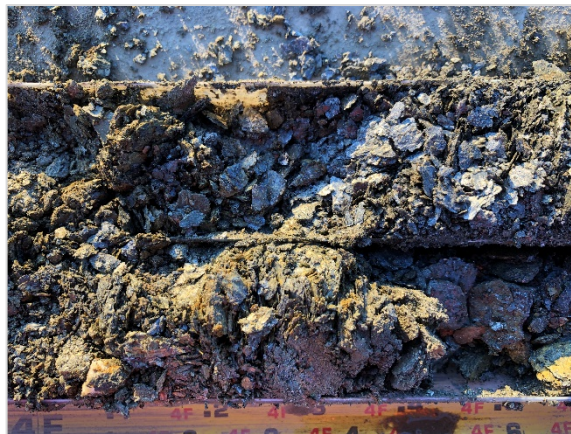
Exhibit 1-3: Schist bedrock encountered in soil boring ARFF-SB3.
