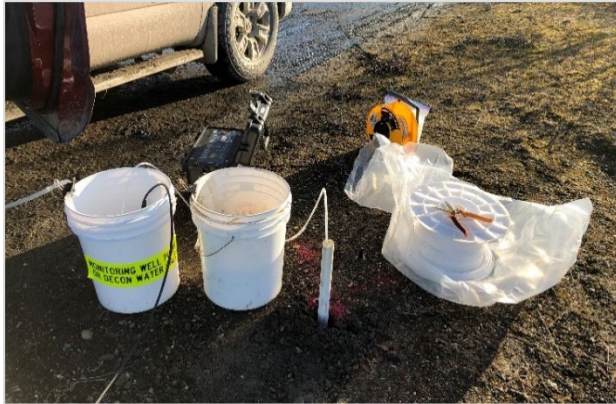
Exhibit 3-3: Groundwater sampling from a TWP
