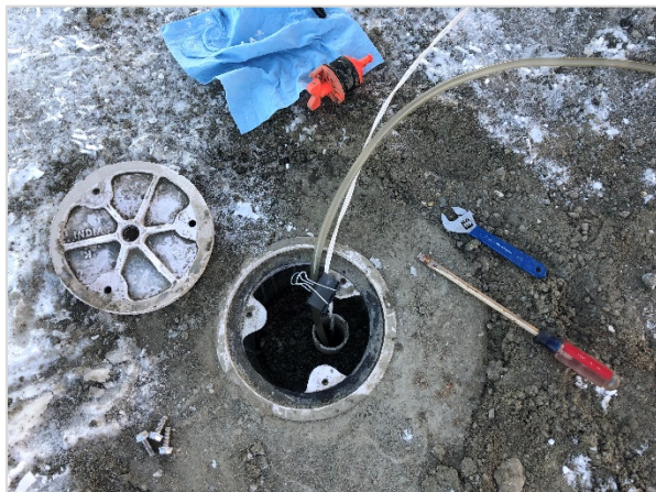
Exhibit 2-3: Groundwater MW sampling
